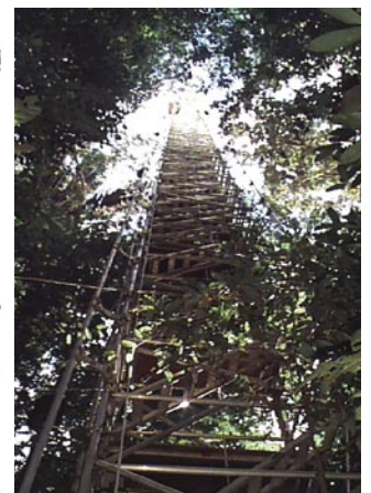
Fig. 5. World-wide distribution of eddy covariance towers measuring CO 2 , water vapour and energy fluxes. Only five such towers were operating 10 years ago. The photo shows an eddy covariance tower near Manaus, Brazil.
